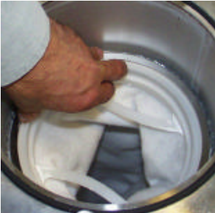
4. Place new filter bag into the basket
