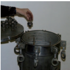
3. Remove spring sealing kits
