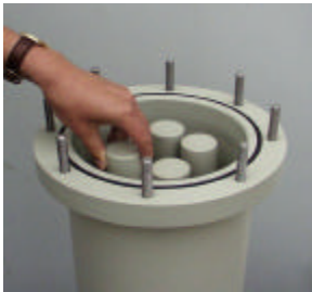
3. Place new filter cartridge on the centre posts and fix element nut by hand
