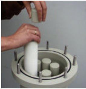
2. Unscrew element nut and pull out filter cartridge
